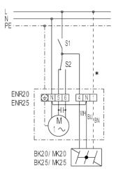
S1 - On / Off S2 - Switching between air extraction and ventilation Terminal 5 - Air extraction Terminal 6 - Ventilation \* - duct only for MK... shutter MK 25
