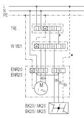
TRE - 5-step transformer (on/off, 5-speed) W 1 - Reversing switch (air extraction or ventilation), surface-mounted WU 1 - Reversing switch (air extraction or ventilation), recessed-mounted \* - duct only for MK... shutter MK 25
