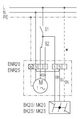
S1 - On / Off S2 - Switching between air extraction and ventilation Terminal 5 - Air extraction Terminal 6 - Ventilation \* - duct only for MK... shutter MK 31
