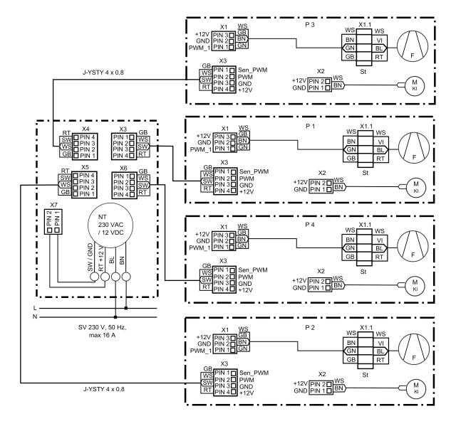
P - PushPull Fan F - Fan KI - Shutter St - Connector NT - Mains adapter SV - Power Supply
