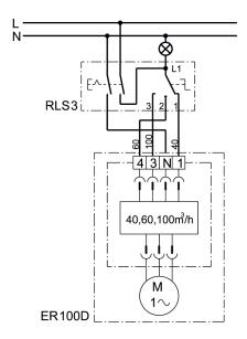
RLS 3 - Room air control with zero position and switch for room lighting
