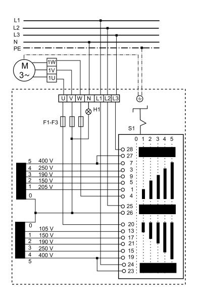
H1 - operation (green) S1 - Switch: On/Off M1 - fan motor (three-phase AC)
