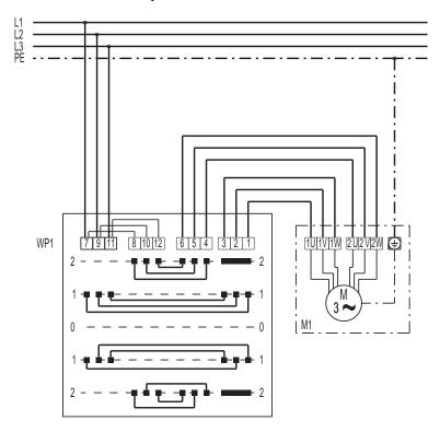
WP1 reversing pole-changing switch: Step 2/Step 1/Off/Step 1/Step 2 M1 fan (Dahlander motor)
