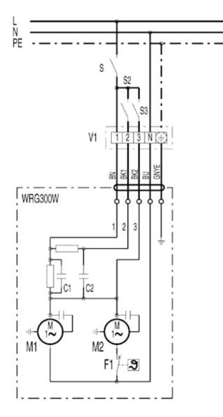
S1 On / Off S2 WRG in level 2 S3 WRG in level 3 V1 distributor (to be provided by the customer) M1 exhaust air fan M2 supply air fan F1 frost protection
