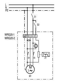
S1 fan On/Off, to be supplied by the customer S2 supply air shutter opening/closing, to be supplied by the customer S4, S5 safety limit switch Z1 supply air shutter M1 fan
