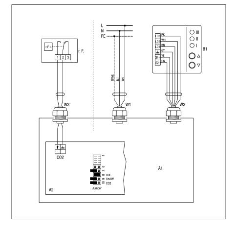
Connection of a hygrostat for demand-driven humidity extraction. This must have a potential-free switching output, e.g. Maico Hygrostat HY 5.
