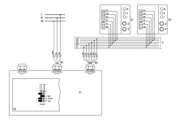
Up to 5 RLS 1 WR room air controls can be connected to the ventilation unit. No CO2 sensor should be connected if several room air controls are connected.
