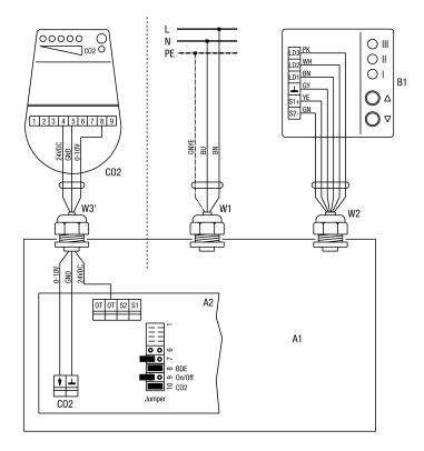
Connection of a CO2 sensor for the demand-driven supply of fresh air. The ventilation unit only reacts to the  $CO_2$  sensor if ventilation level 2 (nominal ventilation) is selected at the room air control.
