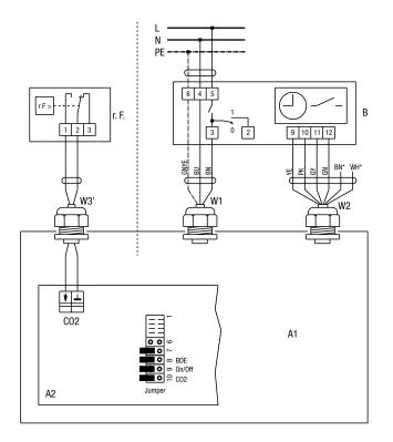
Connection of a hygrostat for demand-driven humidity extraction. This must have a potential-free switching output, e.g. Maico Hygrostat HY 5.
