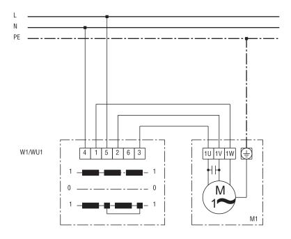
W1 / WU1 - reversing switch: air extraction / off / ventilation M1 - fan (capacitor motor)
