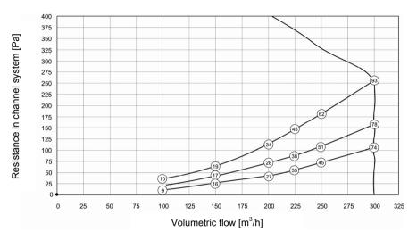
The value in the circle is the power level per fan (in watts).
