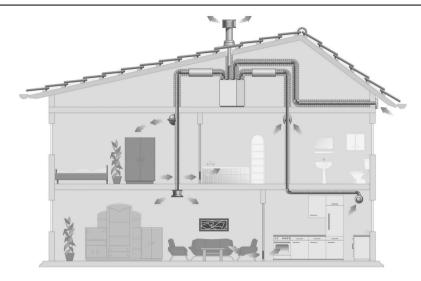
• The outside air feed should be installed on the shaded side of the building, e.g. on the wall or under an overhang. If the outside air is sucked in from underneath the roof tiles, it must be ensured that there is no build-up of condensation in the roof shell and that no water can penetrate. Supply air can be sucked in from underneath the roof tiles if air can flow unhindered from below and above in the roof area and if the building drainage system does not vent out under the roof tiles.
