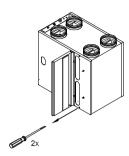
4 Pull the heat exchanger out. Be careful not to damage the foam components in the unit.
