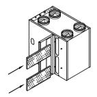
4 Close the filter shutter and switch the unit on at the operating panel by pressing and holding the "OK" and "+" buttons down at the same time for 3 seconds.
