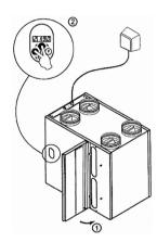
5 The filter status display has to be reset after cleaning or exchanging the filter by pressing the "OK" button for 1 second. The display flashes briefly to confirm and then reverts to operational mode.
