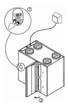
2 Pull the filter out and replace it. Take note of the direction in which the filter was pulled out.
