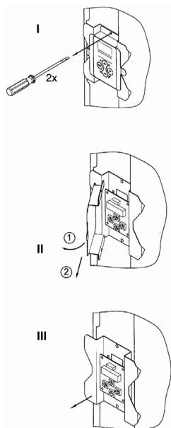
7 Pull out the slider that the main board is mounted on. Remove all connectors from the main board that are connected with the feed through plate. Remove the earthing wire from the housing.
